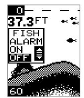
shallower than the alarm's setting. The deep alarm sounds a tone when the bottom goes deeper than it's setting. Both alarms adjust the same, although through different menus.
